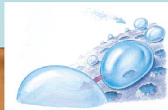
New material that copies the properties of the wing surface of the Namibian desert beetle for collecting precious drinking water from an invisible mist. Inventa Partners: Air Conditioning for recycling water. 2004 (Original research by MIT)
